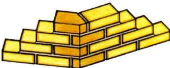
External angle using squint bricks
