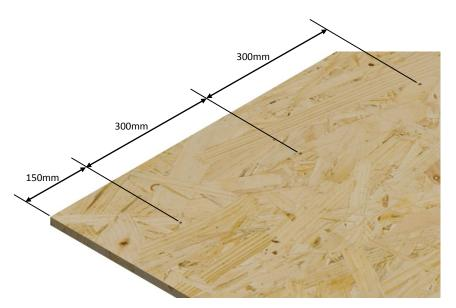
The pre-drilled boards can then be lifted into place and propped if required. The self-drilling and tapping screws are inserted into the clearance holes into the boards and then driven up into the GRP angle to fix the board into position.
